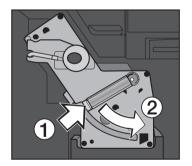
■ Press the light coloured button under the handle of the brew unit ① and whilst doing so turn the handle in the direction of the arrow ②.
